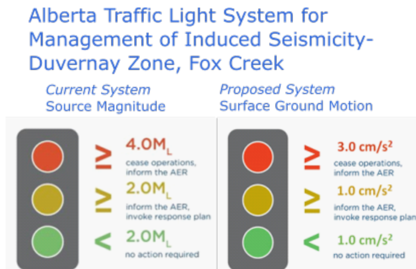
Figure 2. Conceptual overview of the current Traffic Light System for management of induced seismicity, with basis in measuring local source magnitude, and the proposed revised system which would manage surface ground motion (peak ground acceleration) at the nearest affected residence. (After Alberta Energy Regulator 1 )
